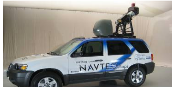
Figure 1. Mobile LiDAR and imagery collection system.
