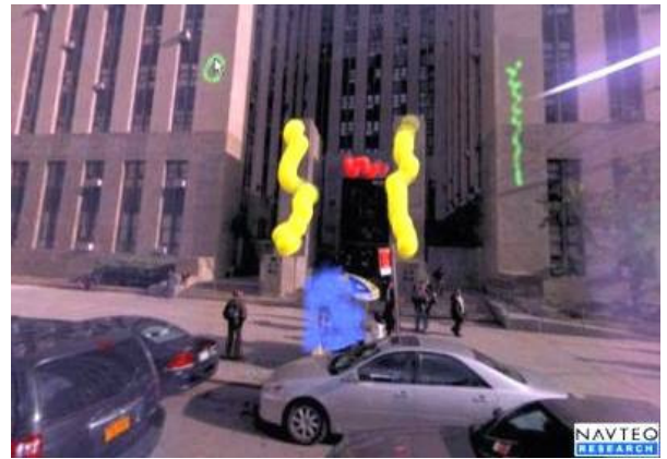
Figure 13. Sketching on 3D objects. Since both the sketch and images are referenced in 3D, the same 3D sketch is valid for other images and viewpoints and is shown with correct perspective scaling. The image depth information is used to determine if the sketch is occluded by objects in the scene (e.g. the car occludes part of the blue sketch).
