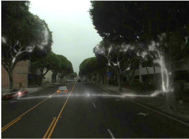
Figure 8. The cross section of a LiDAR point cloud is mixed with the panoramic imagery. This demonstration exposes the 3D structure of the image by moving a cross section through 3D space.
