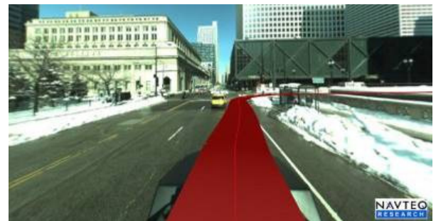
Figure 5. Fixed 3D point focus example. Geo-registered, posed images allow us to automatically look at a fixed world 3D location for any image. In this example, we select a point on the Sears/Willis Tower and step through various images. Our camera always appears to focus on the same fixed point on the building.
