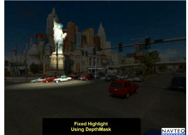
Figure 17. Spot lights alter the panoramic image based on the aligned depth map. User defined spot lights are used to retarget the image brightness based on the light source and each pixel's 3D image depth. In the first case, the user has defined three moving spot lights. In the second case, a top-down spot light is focused on a specific point of interest. Pixels away from the focus position are darkened based on the 3D pixel depth distance from the cone of the light source.
