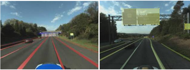
Figure 9. 3D lane marking example, Sign and bridge models are mixed with the panoramic imagery.
