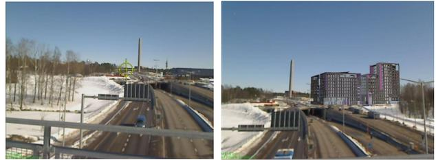
Figure 2. Mobile AR view showing viewfinder for the placemark, and building model augmented with OnSitePlayer.
